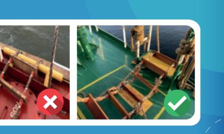
Retrieval lines can be dangerous to both pilots and pilot launches. Retrieval lines pose a trip hazard when climbing and if strung too low may foul the launch. The line **should be** attached above the last spreader and lead forward.
